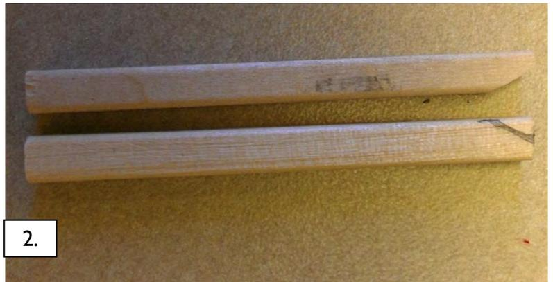
In order to have a reclined backrest you will need to angle the ends of the two  $2 \frac{1}{4}$ " long timbers. Measure  $\frac{1}{16}$ " along the width of each timber and make a small mark. Measure  $\frac{3}{16}$ " from the end of each timber along the length and make a small mark. See illustration 1. Draw a line connecting the two marks. Cut along this line and sand the cut edges. See illustrations 2.
