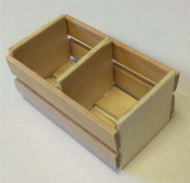
Apply Tacky glue to three edges of the remaining 1" square Woodsie and position this square inside the crate to divide the crate into two compartments. See illustration 5.
