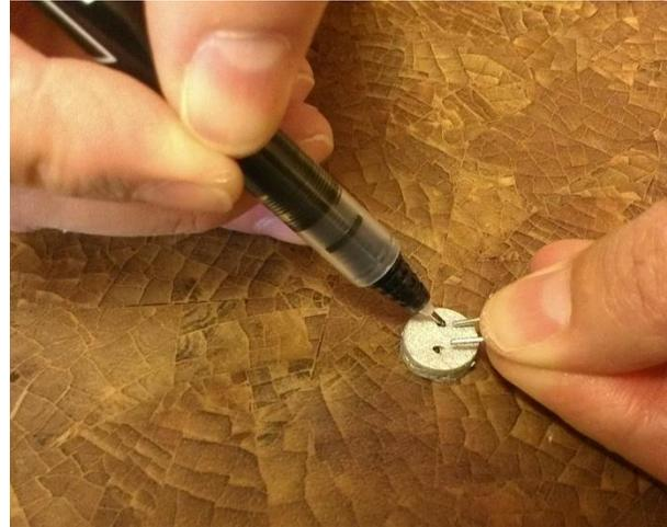
2. Use your permanent marker to mark a hole  $\frac{1}{4}$ " from the top of your vinyl tube and a second hole  $\frac{1}{4}$ " from the bottom edge of the tube. Use the push pin to punch holes all the way through and out the other side of the tube. See illustration 1. Turn the tube 45 degrees, then mark and punch a third hole all the way through the center of the tube. Cut three  $\frac{3}{4}$ " lengths of wire. Thread one wire through each pair of holes to form three perches.
